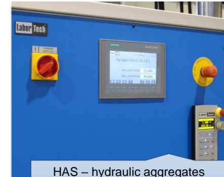
HAS – hydraulic aggregates designed for static tests with integrated diagnostics HALT 18 – Simatic.
